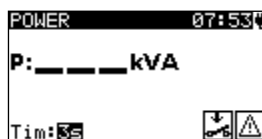
Figure 6.45: Power starting screen
