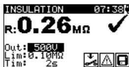
Figure 5.11: Examples of Insulation resistance measurement results
