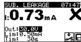
Figure 5.19: Example of substitute leakage current measurement results
