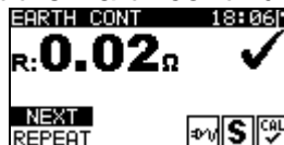
Figure 6.28: Earth continuity result screen
