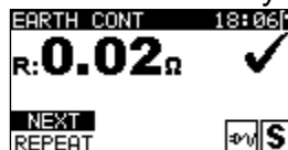
Figure 6.4: VDE Organizer – Earth continuity result screen
