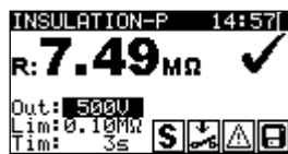
Figure 5.15: Example of insulation resistance - P measurement results
