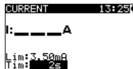
Figure 5.43: Clamp current menu
