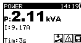
Figure 5.40: Example of apparent power measurement result
