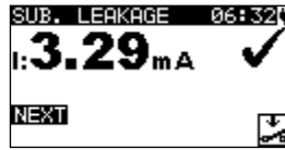
Figure 6.9: VDE Organizer – Substitute leakage result screen
