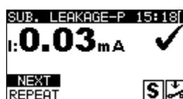
Figure 6.16: VDE Organizer – Substitute leakage - P result screen
