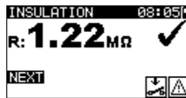
Figure 6.6: VDE Organizer – Insulation resistance result screen
