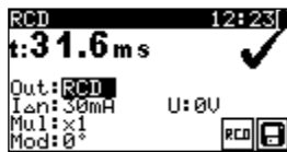
Figure 5.37: Examples of (P)RCD single test results
