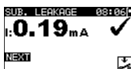
Figure 6.32: Substitute leakage result screen
