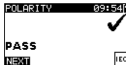
Figure 6.44: Polarity test result screen
