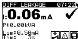
Figure 5.29: Examples of differential leakage current measurement result
