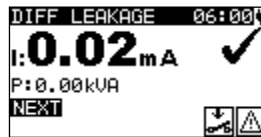
Figure 6.34: Differential leakage result screen
