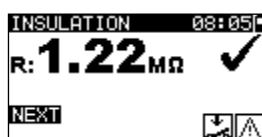
Figure 6.30: Insulation result screen
