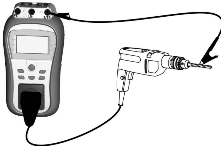
Figure 5.21: Measurement of Substitute leakage - P current
