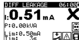
Figure 5.29: Examples of differential leakage current measurement result
