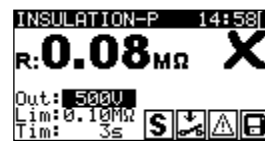
Figure 5.15: Example of insulation resistance - P measurement results
