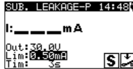
Figure 6.37: Substitute leakage - P starting screen
