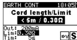
Figure 6.3: VDE Organizer – Earth continuity starting screen
