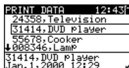
Figure 7.14: Print label / write TAG menu
