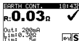
Figure 6.54: Detailed result screen
