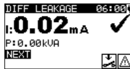
Figure 6.11: VDE Organizer – Differential leakage result screen
