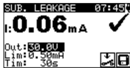
Figure 5.19: Example of substitute leakage current measurement results
