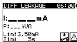
Figure 6.10: VDE Organizer – Differential leakage starting screen
