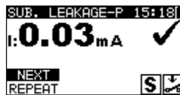
Figure 6.38: Substitute leakage - P result screen
