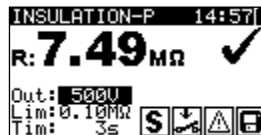
Figure 6.36: Insulation resistance - P result screen
