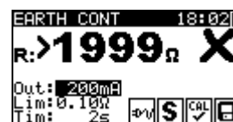
Figure 5.7: Examples of Earth continuity resistance measurement results
