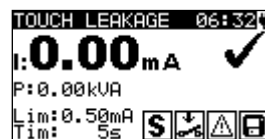
Figure 5.33: Examples of touch leakage current measurement results
